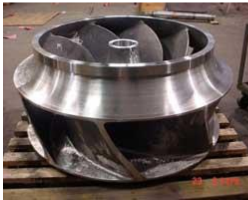
Foster Wheeler 60" Impeller 316 incl. making a pattern; 2150 pounds
