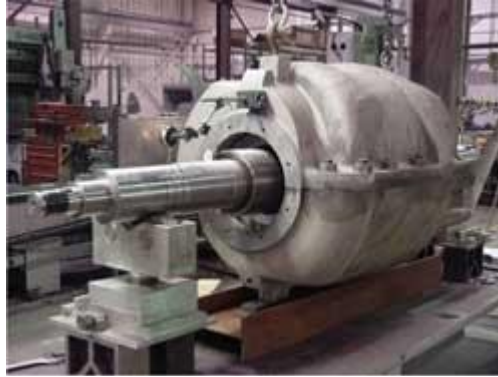
Special Fixture for Final Inspection: Lift / End Float Checks on Boiler Feed Pumps
